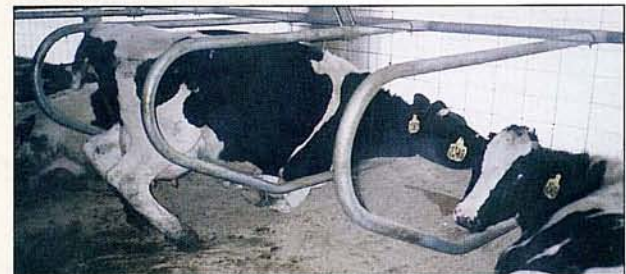
NOTE lunge space available on an outside row using the ALBERS cantilever loop.
